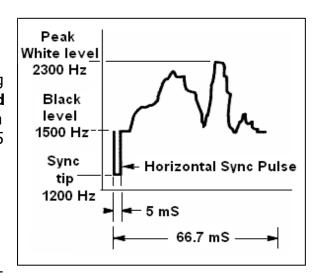
are sent at the end of each line are 5ms in length and at the end of each frame 30ms in length.
