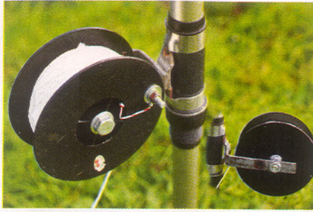
PHOTO 2: How I terminated the wire on the bolt and (inset, right) the bracket I made to fix my homebrew reel to the rod.
